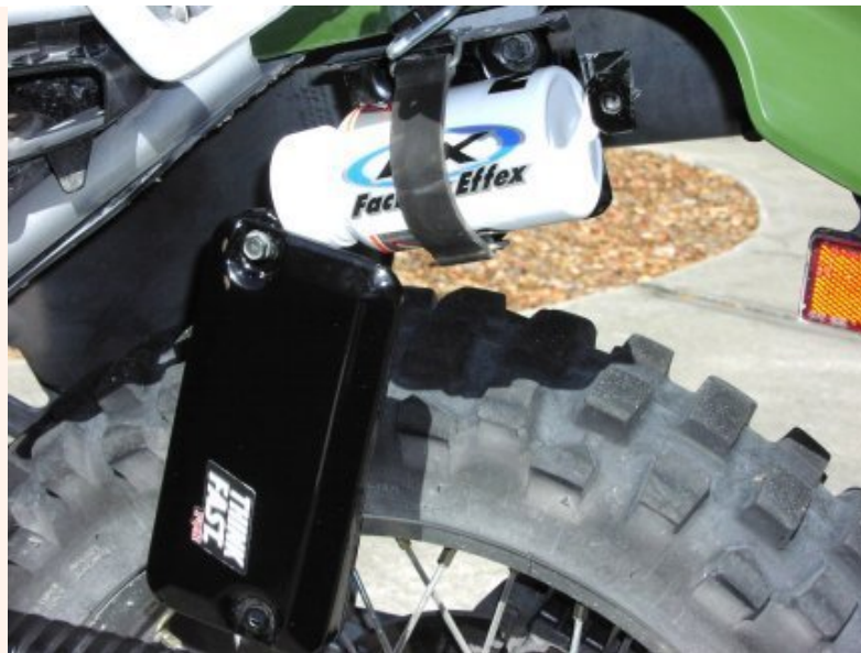
Picture4 above. I used the existing emissions box mounting bracket / hardware / cover, to house a home made, (el cheapo grande), first aid kit. Using the existing emissions canister cover keeps things looking nice & stock.
